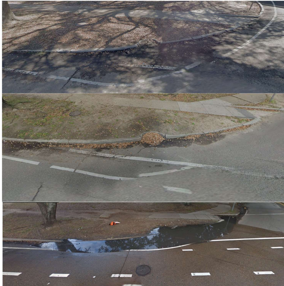
Figure 8: Google Earth 2011 to 2025 Imagery of Clogged Inlet at St. Bernard and N. Claiborne
